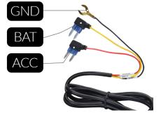
BAT – Yellow cable BAT+ connects to a fuse holder that always supplies power, even when the vehicle is off.
