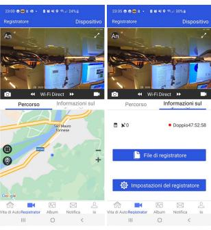
The app allows you to control the front and rear cameras. With the small An/P button on the top left you can select the camera. With the camera and video buttons located below the image you can take photos and record videos to save on your phone.
