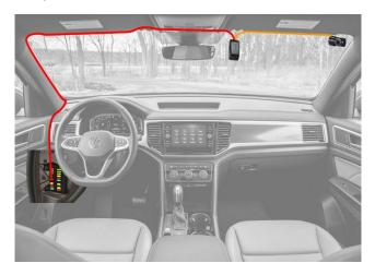
Example with installation of second internal (A) or external (B) rear camera
